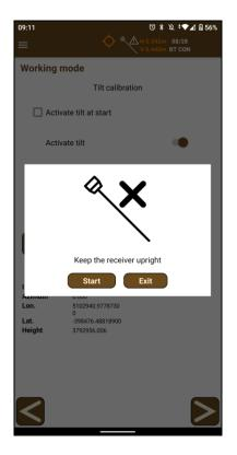
Figure 9. Tilt calibration dialog
