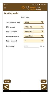
Figure 3. UHF Base working mode
